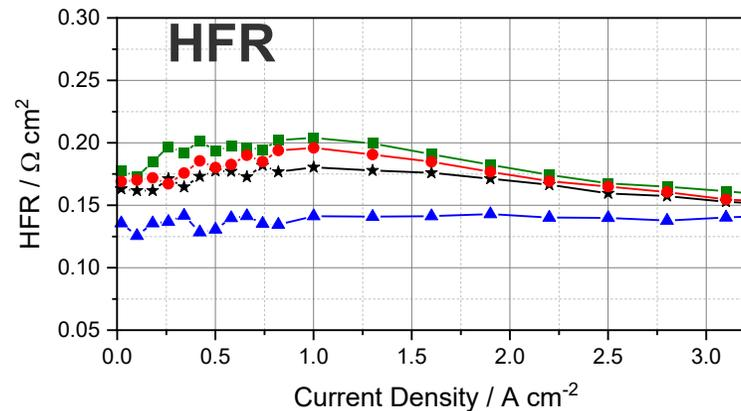
Cell Temperature: 80 °C; Flow rate: 50 ml min<sup>-1</sup>; Active area: 25 cm<sup>2</sup>; Anode: 0.1 mg cm<sup>-2</sup> IrO<sub>2</sub> (Alfa Aesar); Cathode: 0.1 mg cm<sup>-2</sup> Pt/C; PTL: 2GDL10
