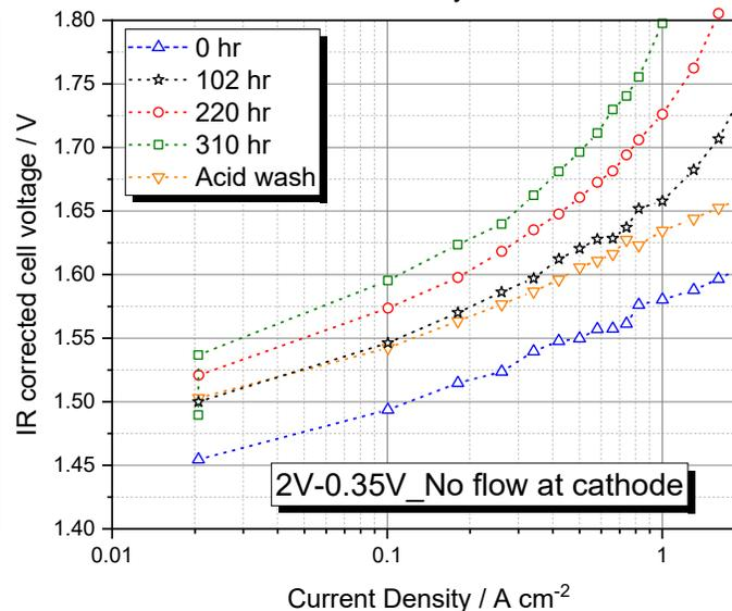
Cell Temperature: 80 °C; Flow rate: 50 ccm; Active area: 25 cm<sup>2</sup>; Anode: 0.1 mg cm<sup>-2</sup> IrO<sub>2</sub> (Alfa Aesar) ; Cathode: 0.1 mg cm<sup>-2</sup> Pt/C; PTL: 2GDL10
