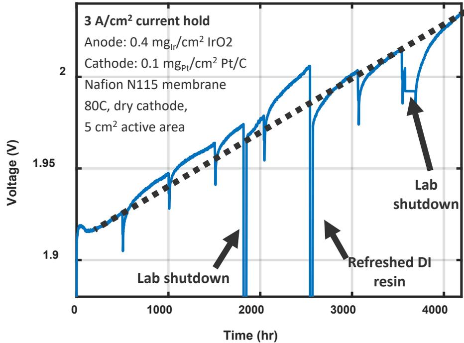
Completed 4,000 hr durability test of FuGeMEA cell:
