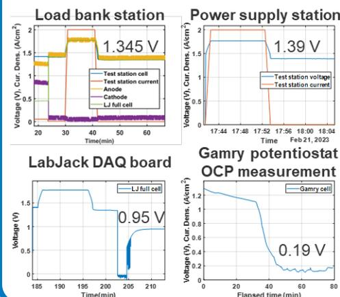
**Experimental Challenge Identified:** Stray currents from test station, potentiostat, or voltage measurement devices can influence shutdown conditions and reference electrode measurements.
