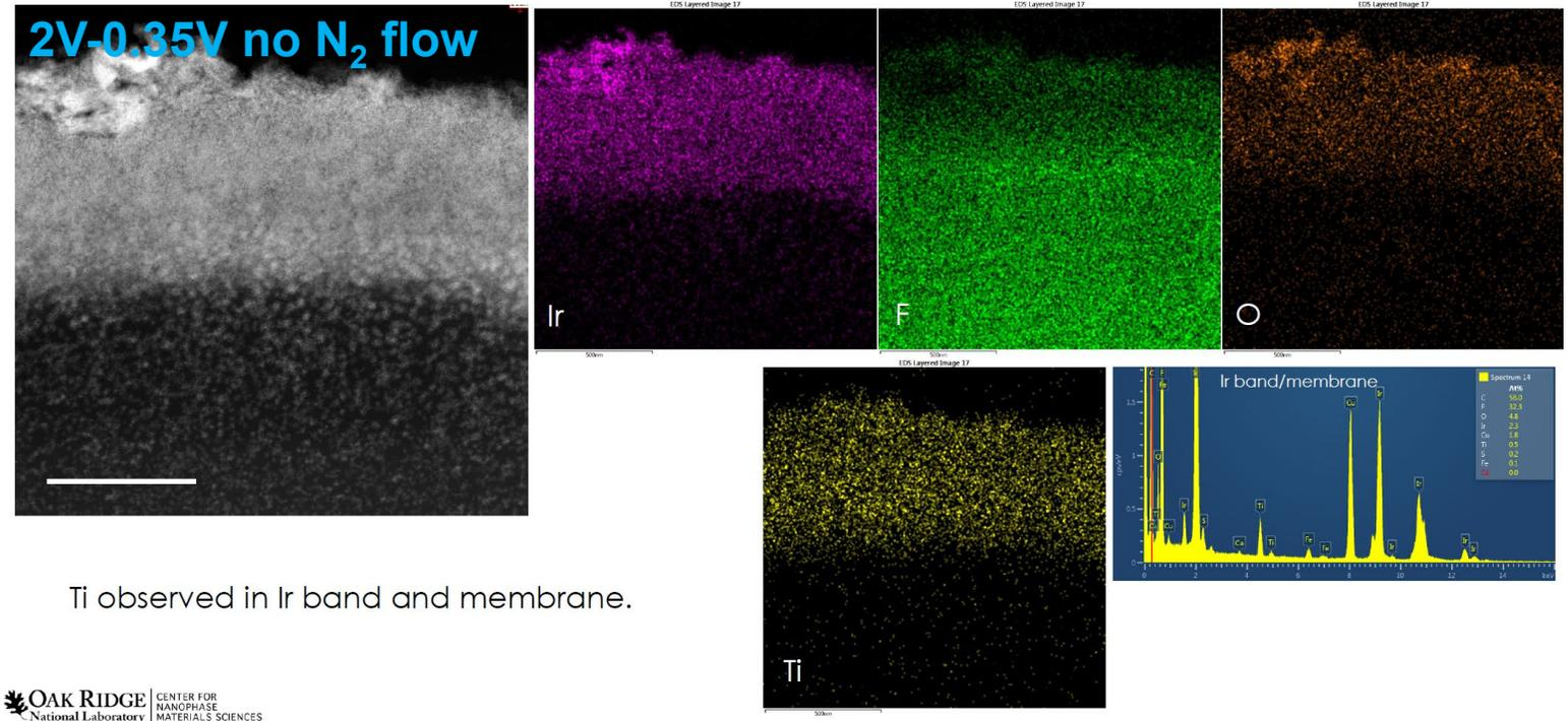
Ti observed in Ir band and membrane.
