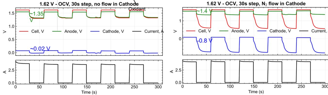
➤  $N_2$  purging the cathode increases cell durability by increasing the anode potential and decreasing the cathode potential enabling a more stable environment for both electrodes' catalysts.
