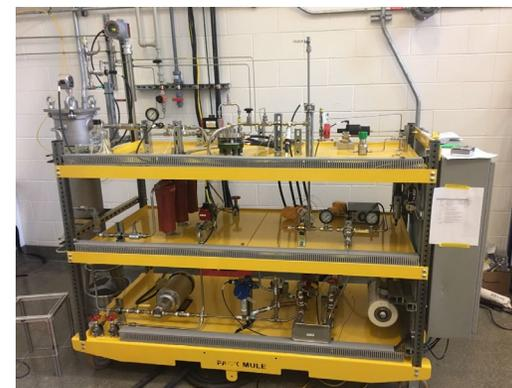
Side view of the short stack testing platform at NREL. This highly automated system can monitor BoP and stack performance during stack durability testing.
