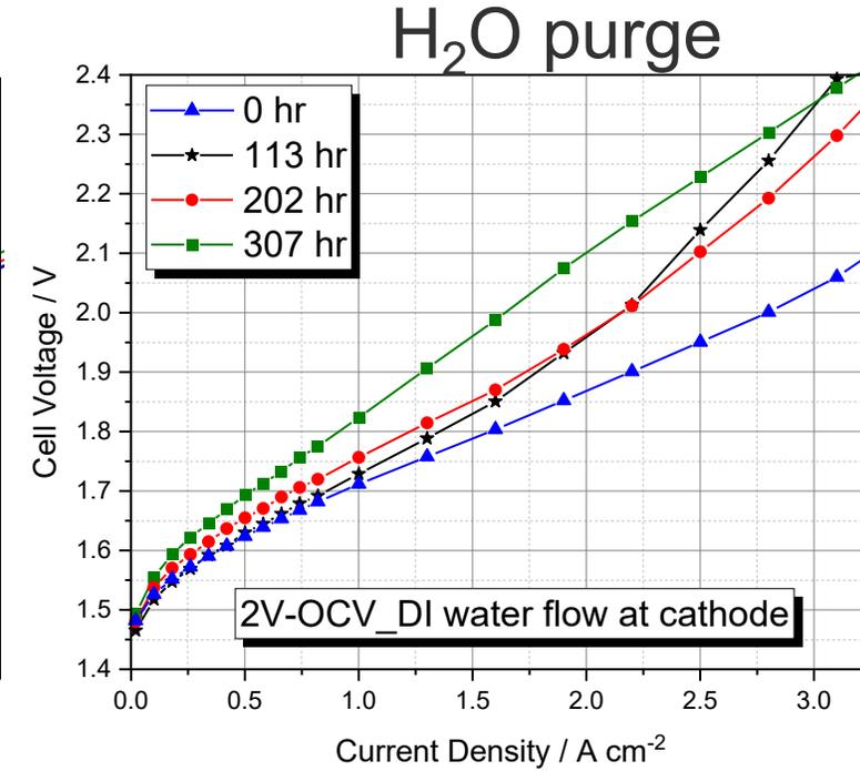
Cell Temperature: 80 °C; Flow rate: 50 ml min<sup>-1</sup>; Active area: 25 cm<sup>2</sup>; Anode: 0.1 mg cm<sup>-2</sup> IrO<sub>2</sub> (Alfa Aesar); Cathode: 0.1 mg cm<sup>-2</sup> Pt/C; PTL: 2GDL10
