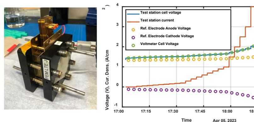
Measurement of anode and cathode potentials to identify depolarization mechanism and stressors during shutdown.
